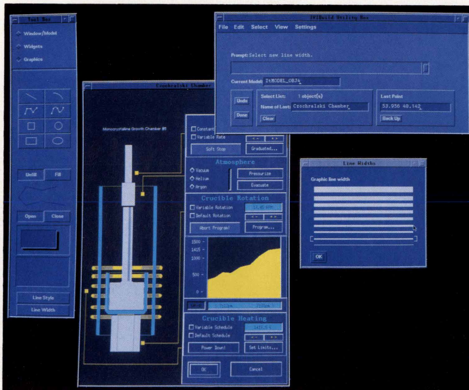
Fig. 2. An application user interface being created using the interactive tools provided by HP IVIBuild. The tool box, utility box, and line width panels are HP IVIBuild components.
